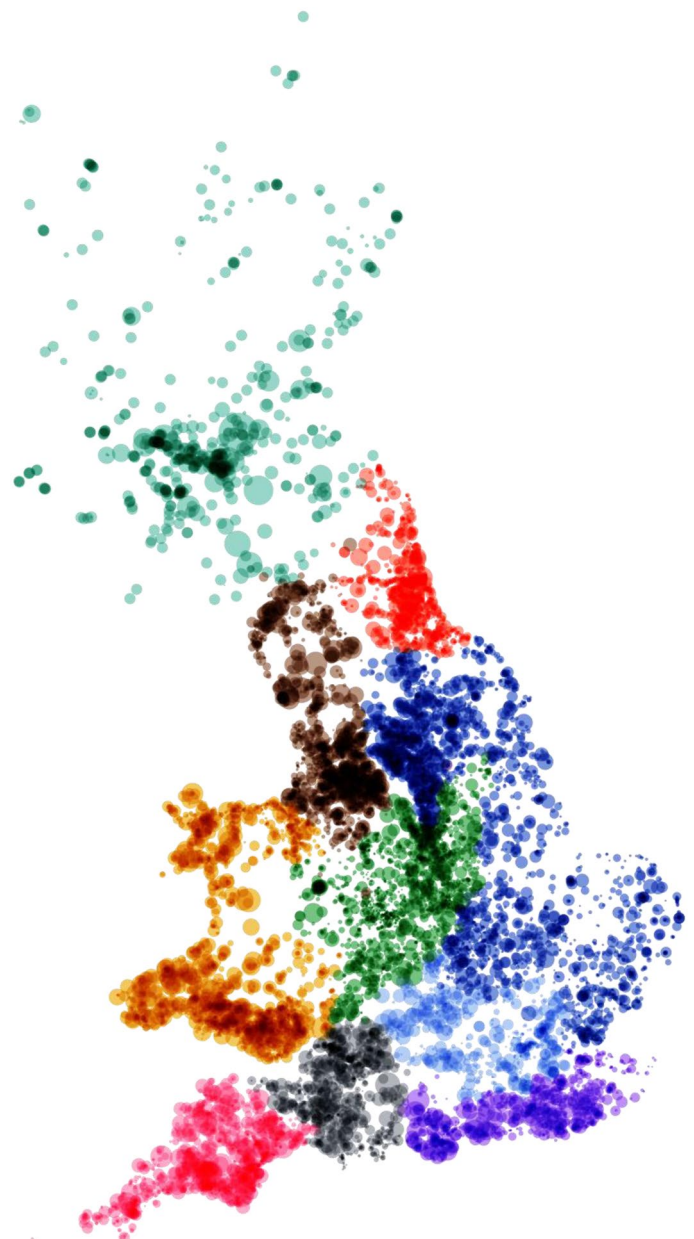
Fig. 1 | CSO duration for 2023. Circles show individual overflows, with the size being proportional to duration (0–8,700 h) and the colour differentiating the WaSCs. Figure adapted from Top of the Poops under a Creative Commons license CC BY-SA 4.0.
